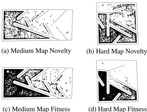
Figure 4: **Final Points Visited Over Typical Runs.** Each maze depicts a typical run, stopping at either 250,000 evaluations or when a solution is found. Each point represents the end location of a robot evaluated during the run. Novelty search is more evenly distributed because it is not deceived.
